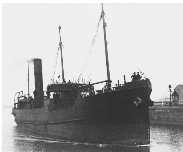
ss Camlough . She was a typical engines aft, central exposed bridge, two hatch vessel
