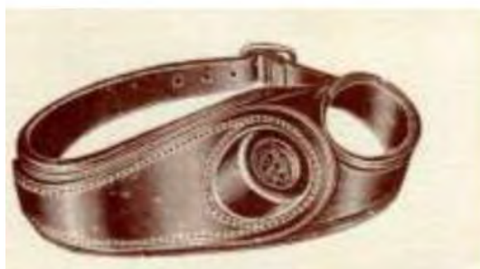
No. 5 Adjustable leather seaming palm, half-lined around thimble.
