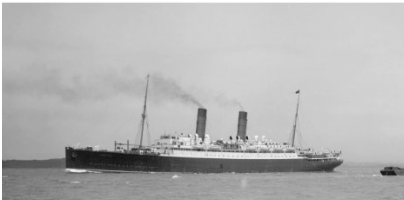
RMS Franconia was launched 23 July, 1910 by Swan, Hunter & Wigham Richardson of Tyneside. Of 18,150 g.r.t. with a length of 625ft., beam of 71ft. she carried 2,850 passengers. Powered by quadruple expansion engines and two propellers she operated at a service speed of 17 knots
