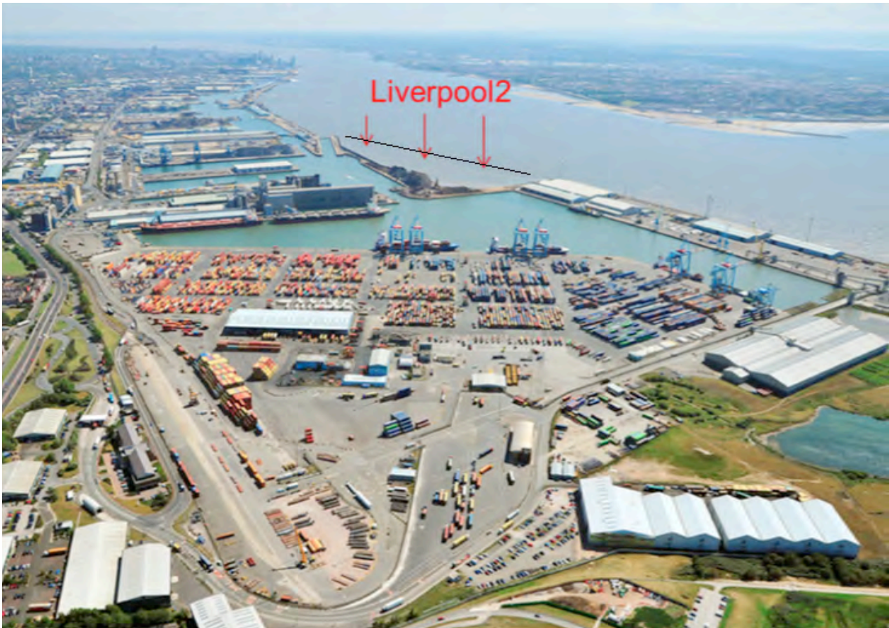
The arrows point to Phase 1 of the development, the infill of a triangular area to form the apron of the new berths and location of the eight quay cranes
