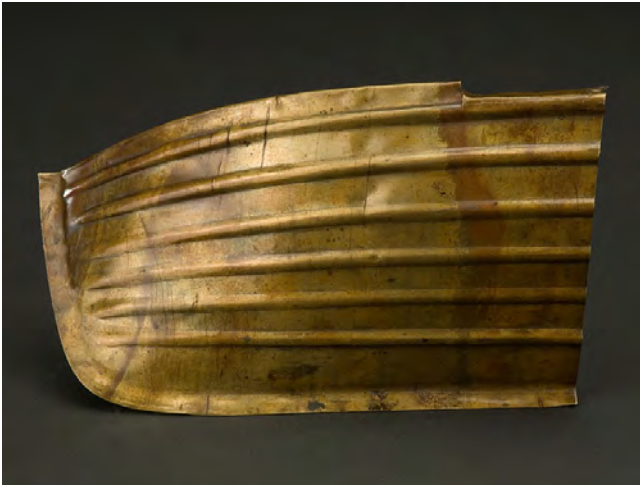
Francis also donated models of dies, and this sample copper sheet formed on them, to the Smithsonian in 1885.
